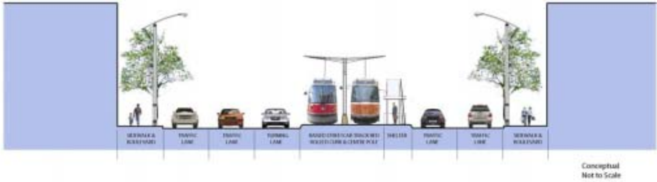
Figure 21: Conceptual cross-section of Preferred Alternative at Bathurst Street intersection, featuring raised trackbed with rolled curb, center pole and transit shelter.
