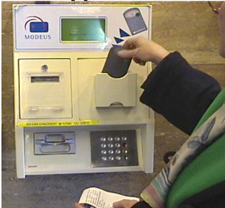
Customer recharging RATP's smart card at a Bank ATM
